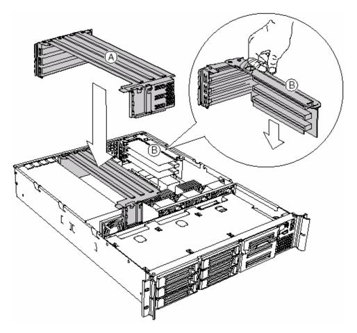
Figure 24: Installing a Riser Card
